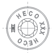
Head markings for d = 7.0 bis 10.0 mm all head types Head types without lettering possible.
